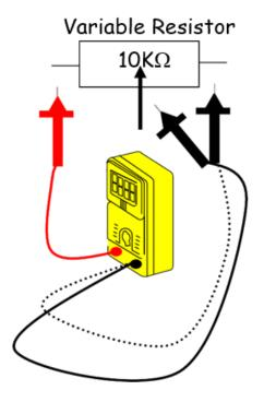
Variable resistors may be used on manual feed guides, varistors, cassette size detect i.e. paper width.
