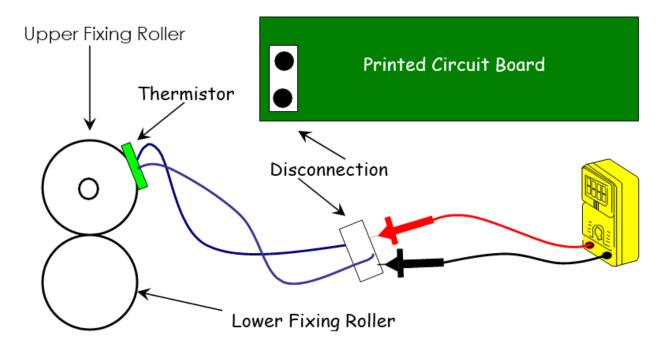
When checking the thermistor always avoid finger contact with the probe points or terminals being tested as this will allow for 'body resistance' readings and thus generate false readings. The resistance being measured will change as the thermistor cools. It is interesting to note that the resistance value is not an important issue as long as consistent variation in resistance is measured during cooling of the upper fixing roller.
