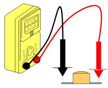
Insulated wire and solid conductors should of course provide a suitable path for current flow, in whatever application. The wiring or conductors can be checked for continuity. 'Tracks' on a circuit board can also be tested for continuity. The machine earth integrity is, as every field service technician knows a mandatory routine test (i.e. the metal framework of the product to the earth pin of the mains plug).
