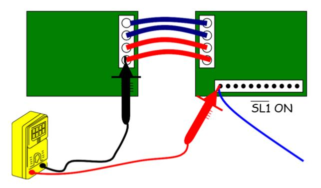
This method positively indicates the 'truth' of the active low signal and avoids the risk of false indication caused by the momentary loss of connection between probe and test point when using 0 volt as a reference.
