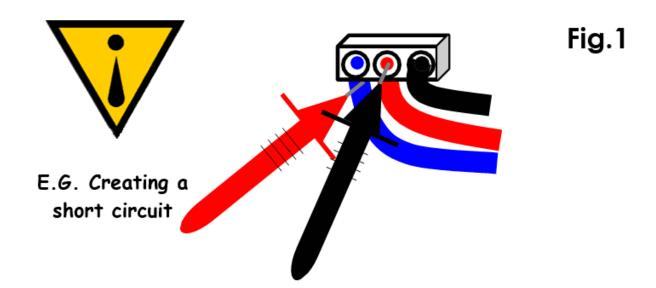
When faced with the situation as previously mentioned in Fig 1. perhaps a more distant reference should be used for example when measuring a high active signal. It is possible to find another 0 volt reference which guards against the close proximity of meter probe tips as demonstrated on page 18.
