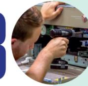
The machine is then reassembled on a factory standard production line, using existing as well as new parts. Hard drives are erased and reformatted and the machine is upgraded with the latest applicable firmware. The counters are set to zero, the machine is assigned a new serial number and given a brand-new factory warranty.
