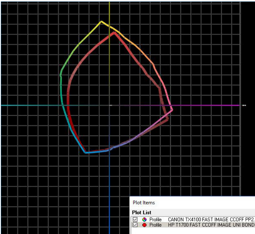
Canon imagePROGRAF TX-4100 colour gamut on plain paper in Fast settings (shown chromatically) versus HP DesignJet T1700dr colour gamut (shown in red) on plain paper in Fast settings.
