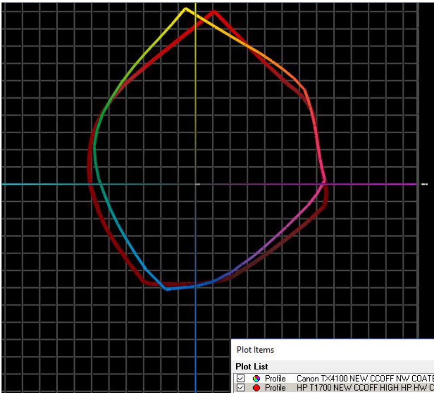
Canon imagePROGRAF TX-4100 colour gamut on matte coated paper in High quality settings (shown chromatically) versus HP DesignJet T1700dr colour gamut (shown in red) on matte coated paper in Best settings.
