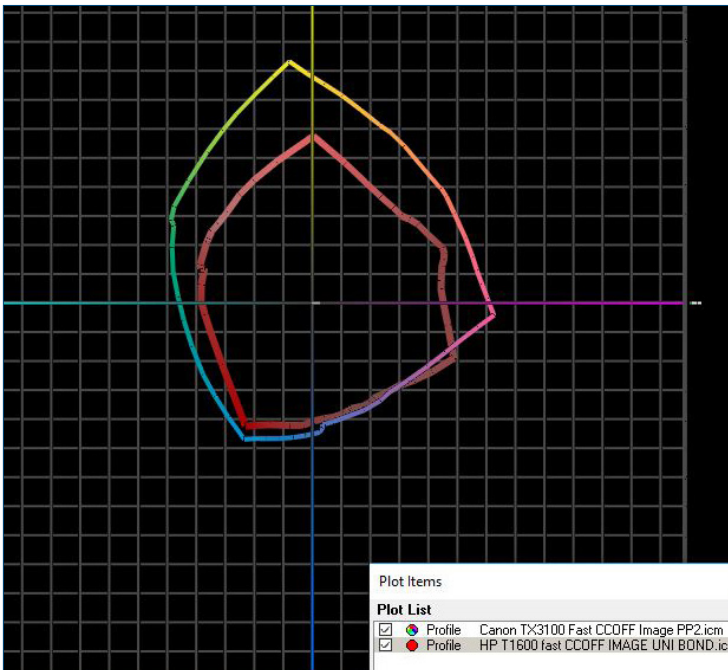
Canon imagePROGRAF TX-3100 colour gamut on plain paper in Fast settings (shown chromatically) versus HP DesignJet T1600dr colour gamut (shown in red) on plain paper in Fast settings.
