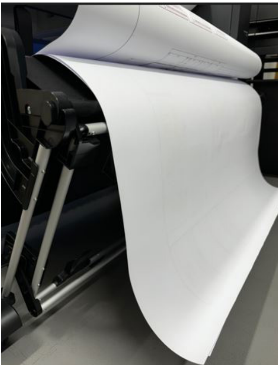
Canon imagePROGRAF TM-350's catch basket holding A1-size prints (top) and A0-size prints (bottom).
