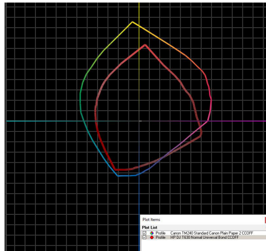
Canon imagePROGRAF TM-240 colour gamut on plain paper in Standard settings (shown chromatically) versus HP DesignJet T630 colour gamut (shown in red) on plain paper in Normal settings.
