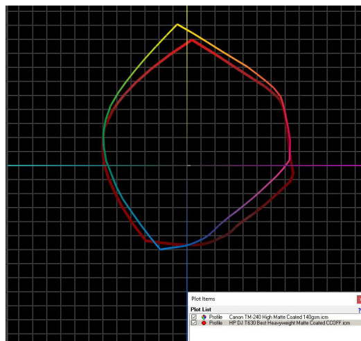
Canon TM-240 colour gamut on matte coated paper in High quality settings (shown chromatically) versus HP DesignJet T630 colour gamut (shown in red) on matte coated paper in Best settings.
