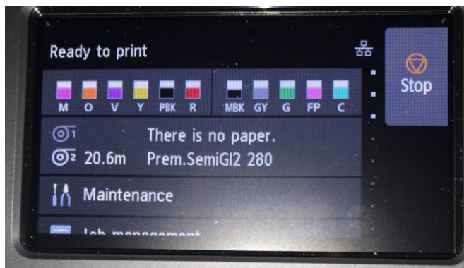
Canon GP-4000's Control Panel
