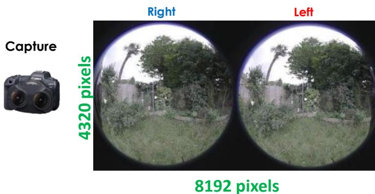
The stereoscopic fisheye images are captured by one sensor onto a single file. Right and left lens images are initially captured in reverse order, as viewed on the camera's LCD screen.
