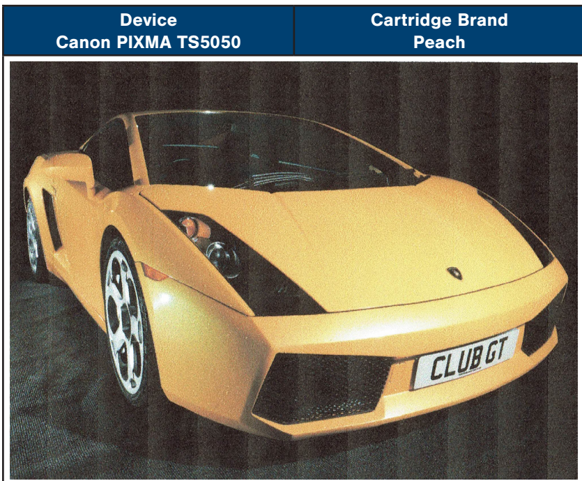
500 impressions, severe defect The banding in this image is so apparent that it ruins the image; the banding detracts the viewer's attention from the image and affects the colours.
