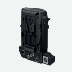
Extension Unit 3 EU-V3 Built for live multi-cam productions, this EU-V3 Expansion Unit adds Return SDI Signal Input, Tally Signal Support, 12-pin Lens Terminal, Remote B (RS-422), and more.
