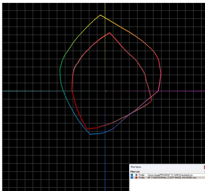
Canon imagePROGRAF TX-3200 colour gamut on plain paper in Standard settings (shown chromatically) vs. HP DesignJet T1600dr colour gamut (shown in red) on plain paper in Normal settings.
