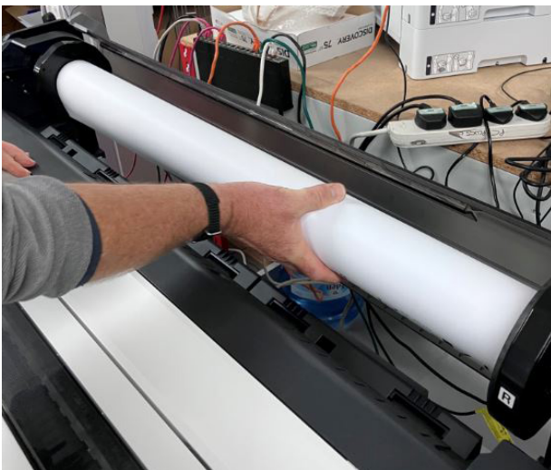
Roll media is loaded onto a spindle for both devices (Canon, left; HP, right)
