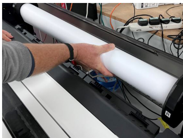
Roll media is loaded onto a spindle for both devices (Canon, left; Epson, right)
