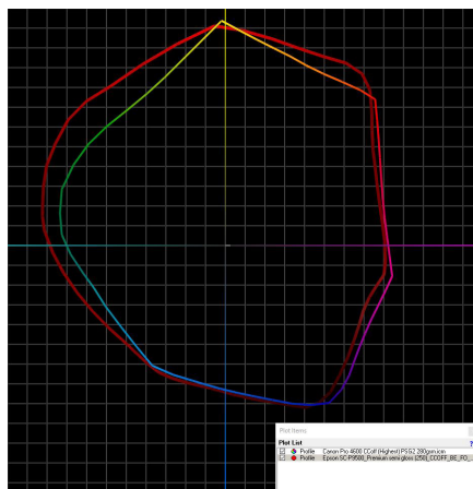
Canon imagePROGRAF PRO-4600 colour gamut (shown chromatically) on semi-gloss photo paper in Highest mode with colour correction disabled versus Epson SureColor SC-P9500 colour gamut (red) on semi-gloss photo paper in Max Quality mode with colour adjustment disabled.
