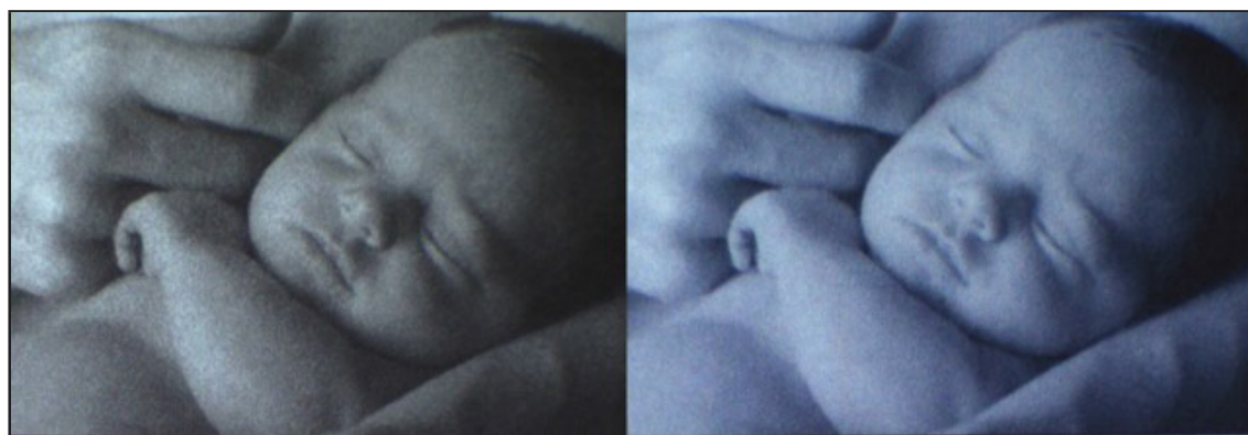
MAXIFY GX4050 output (left) against EcoTank ET-4850; more accurate shade of gray, while Epson output appears overly blue with a cooler color temperature.
