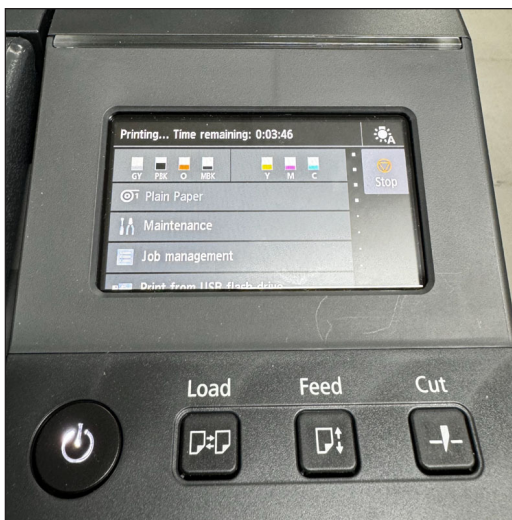
Canon GP-4600S control panel
