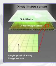
Thanks to the new real-time pixel readout technology, the new Canon detector is able to generate a signal to the generator when sufficient dose is received without the conventional technology to achieve the optimal dose versus image quality balance
