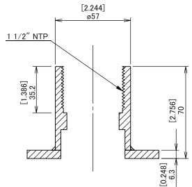
Coupling for Dome Housing & 1 1/2"NPT
