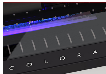
Low heat LED UV curing process, prevents media distortion.
