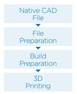
The process starts with the 3D CAD file which needs to be reproduced. This can come from a variety of sources including 3D scan data and new 3D CAD designs. Most modern 3D modelling packages provide interfaces and output formats which are compatible with 3D print software.
