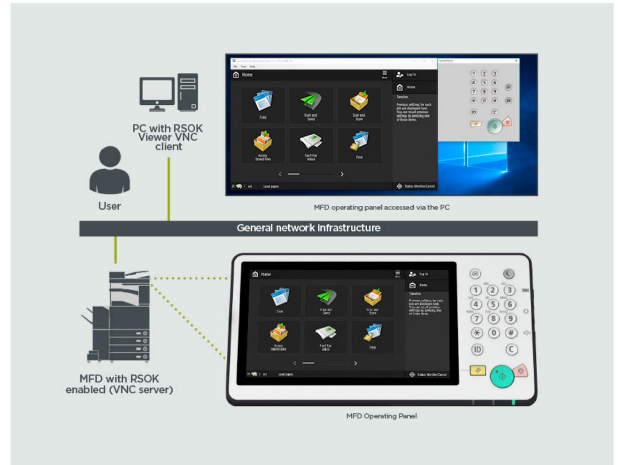
**Figure 12** Remote Support Operator's Kit (RSOK) Setup
