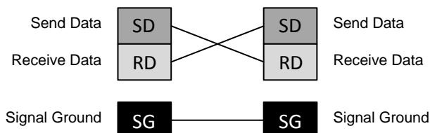
\* Signal lines other than the three SD, RD, and SG lines are not used in the projector.
