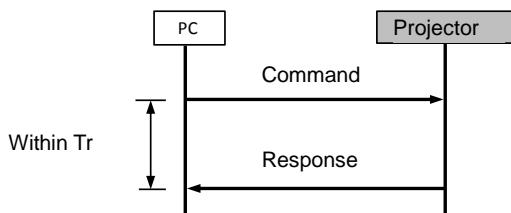
(\*) The timeout interval between command and response (Tr) is 15 seconds.
